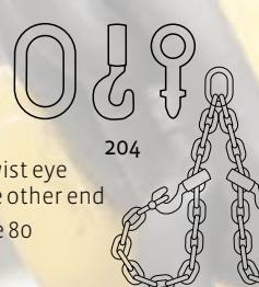
**Description:** Masterlink in one end, twist eye chooke on the chain, omega link in the other end
