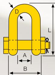
**D-Ring, svetsbar / Weld on Lifting Point**
