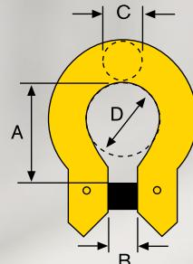
**Rundslingskoppling / Web Sling Connector**
