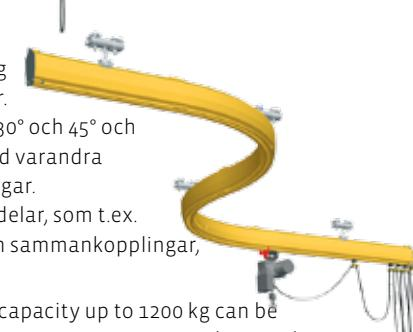
Hoist tracks with a load capacity up to 1200 kg can be fitted with curves. The curves are as 15°, 30° and 45°, and can be freely combined with each other using standard joints. Other advanced parts such as table turns, switches and interconnects, are available.
