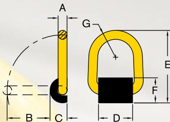
**Grävmaskinskrok / Exavactor Weld-On Hook**
